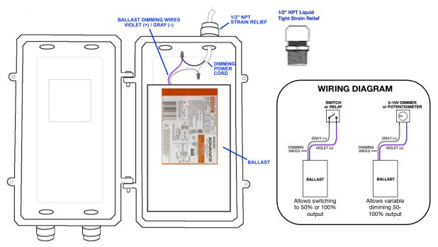
After installation, carefully close the ballast enclosure, making sure no wires are pinched.
